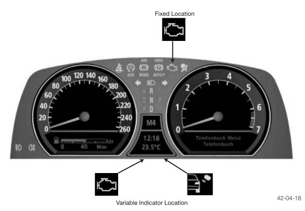
The Malfunction Indicator Light will illuminate with a "half shading" in the variable indicator location for the following reasons:
